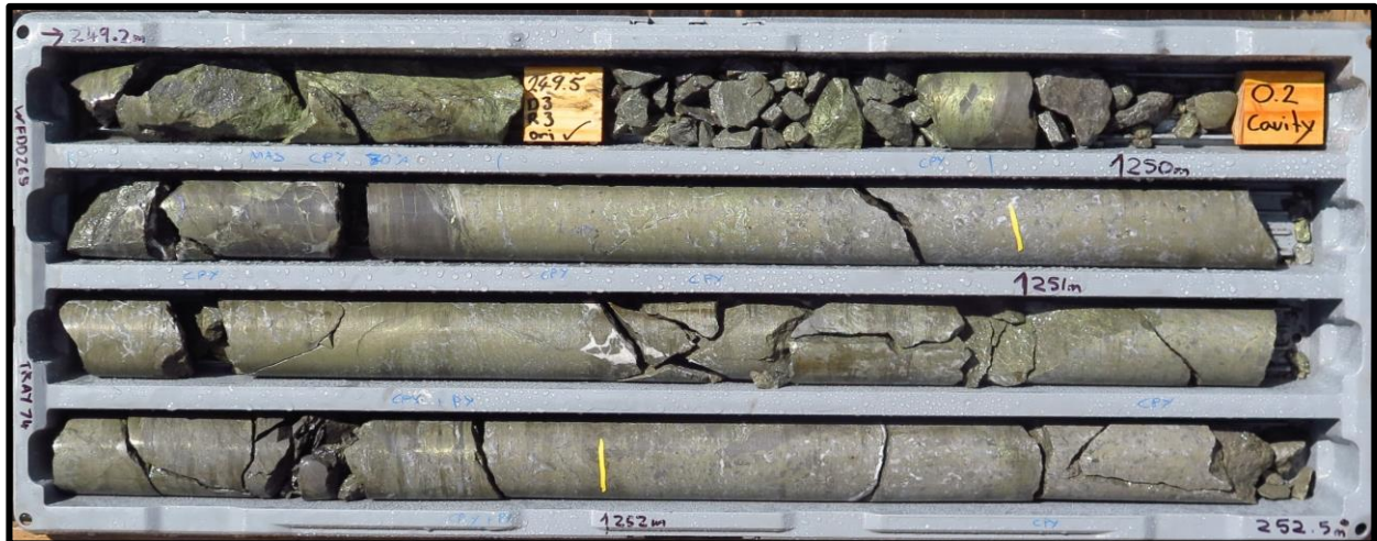
Figure 1: Tray 74 from hole WFDD265 just completed. Strong chalcopyrite mineralisation evident overprinting pyrite zones in micrite dolomite unit at roughly 250m in Py3 at Walford Creek.
