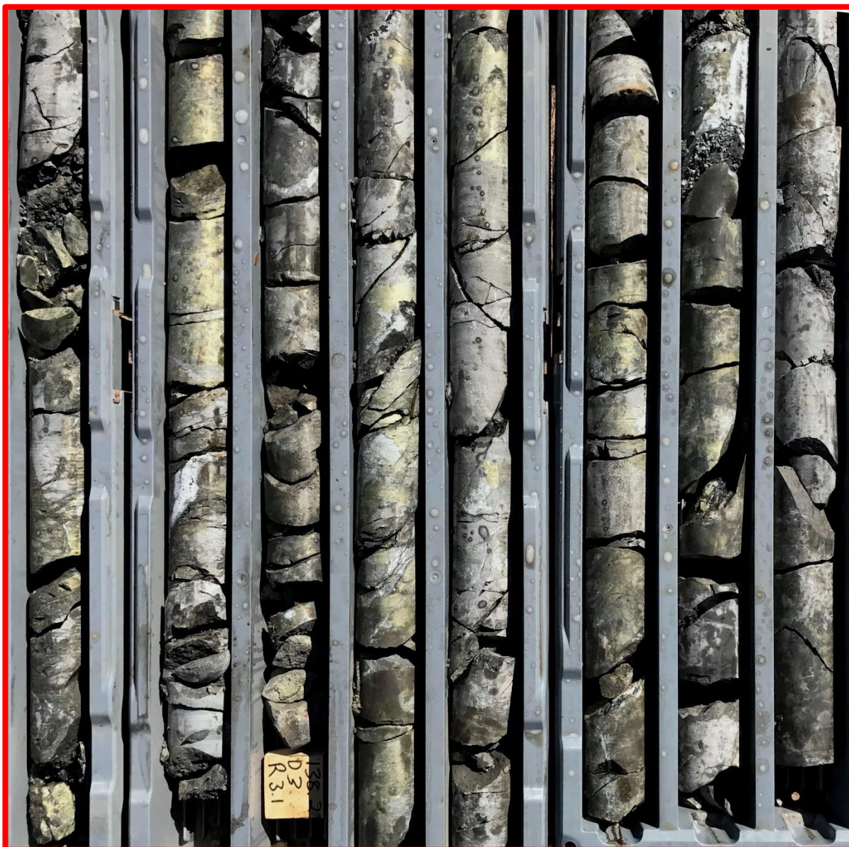
Figure 2: Core from WFDD239 within the Vardy zone and now in Mt Isa awaiting cutting prior to analysis. Strong chalcopyrite mineralisation within the brecciated dolomitic siltstone shale sequence of the Mt Les siltstone.
