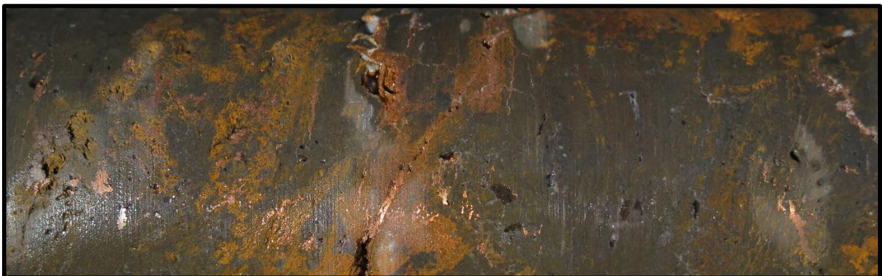
Figure 1: WFDD221 Native copper from 54.8m downhole. Core photographed is HQ diameter and 12cm long.
