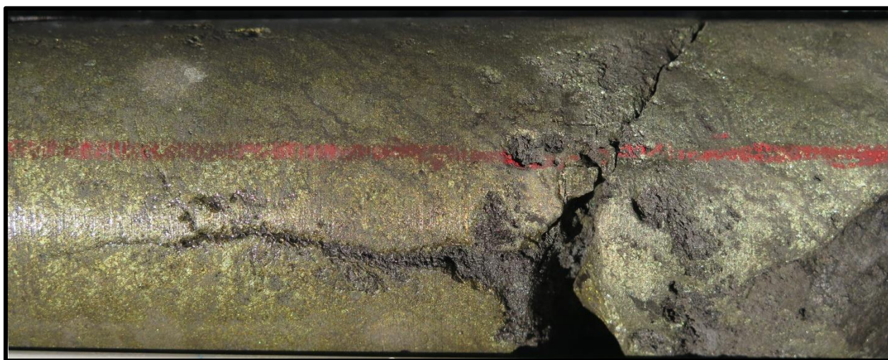
Figure 3: WFDD223 showing semi massive chalcopyrite at 75.5m downhole. This hole was the last and eastern most hole of the September drill program. Core photographed is HQ diameter and 10cm long.
